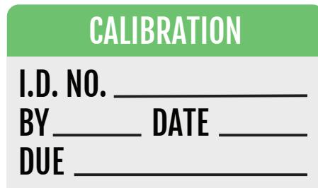
**I.D. NO.** - This will be the identification number assigned to the tool. This number will be used for tracking purposes in the tool system.
