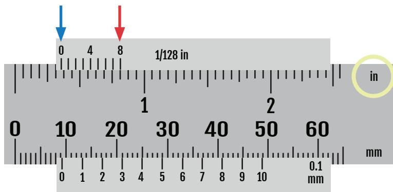
To measure in inches, locate the inches side of the caliper scale based on the “in” marking (circled in yellow).
