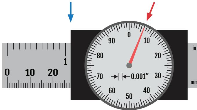
Choose a unit system to measure in whether it be metric (mm) or imperial (in). If you using the metric system, only the main scale of the caliper is used. If using imperial, the main scale and dial will be used.
