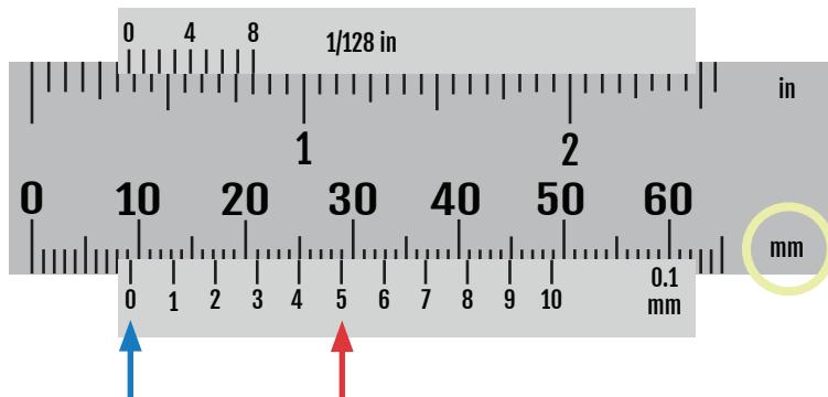
To measure in milimeters, first locate the milimiters side of the caliper scale based on the “mm” marking (circled in yellow).
